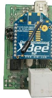
(b) XBee Series 2 Gateway Adapter
