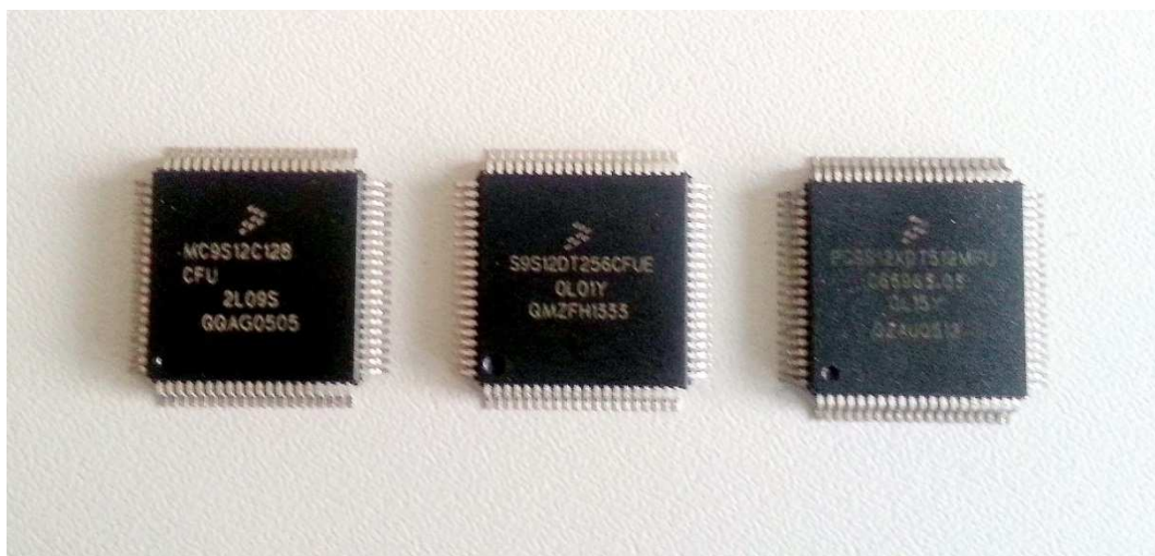
Figure 1.1 The three S12 cores included in the ZK-S12-B kit: S12C128, S12DT256 and S12XDT512 (with XGATE co-processor)
