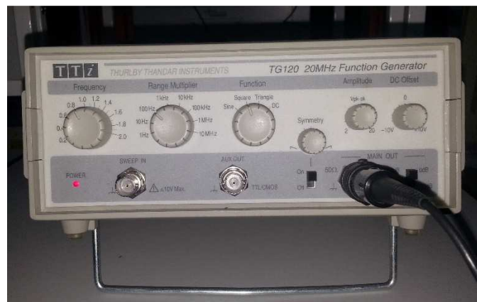
Figure 7.3 TG120 function generator (use it to generate the square wave that is the input to the ADC)
